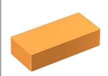
Brick n.1 Category b: Solid clay masonry: Bulk density class  $\rho$ =1.6 kg/dm<sup>3</sup> Minimum compressive strength fb=18 MPa
