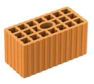
Brick n.2 Category c: Hollow masonry: Bulk density class  $\rho$ =0.9 kg/dm<sup>3</sup> Minimum compressive strength fb=6.0 MPa
